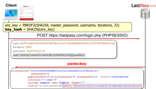
Fig. 4. Client-server communications of LastPass
